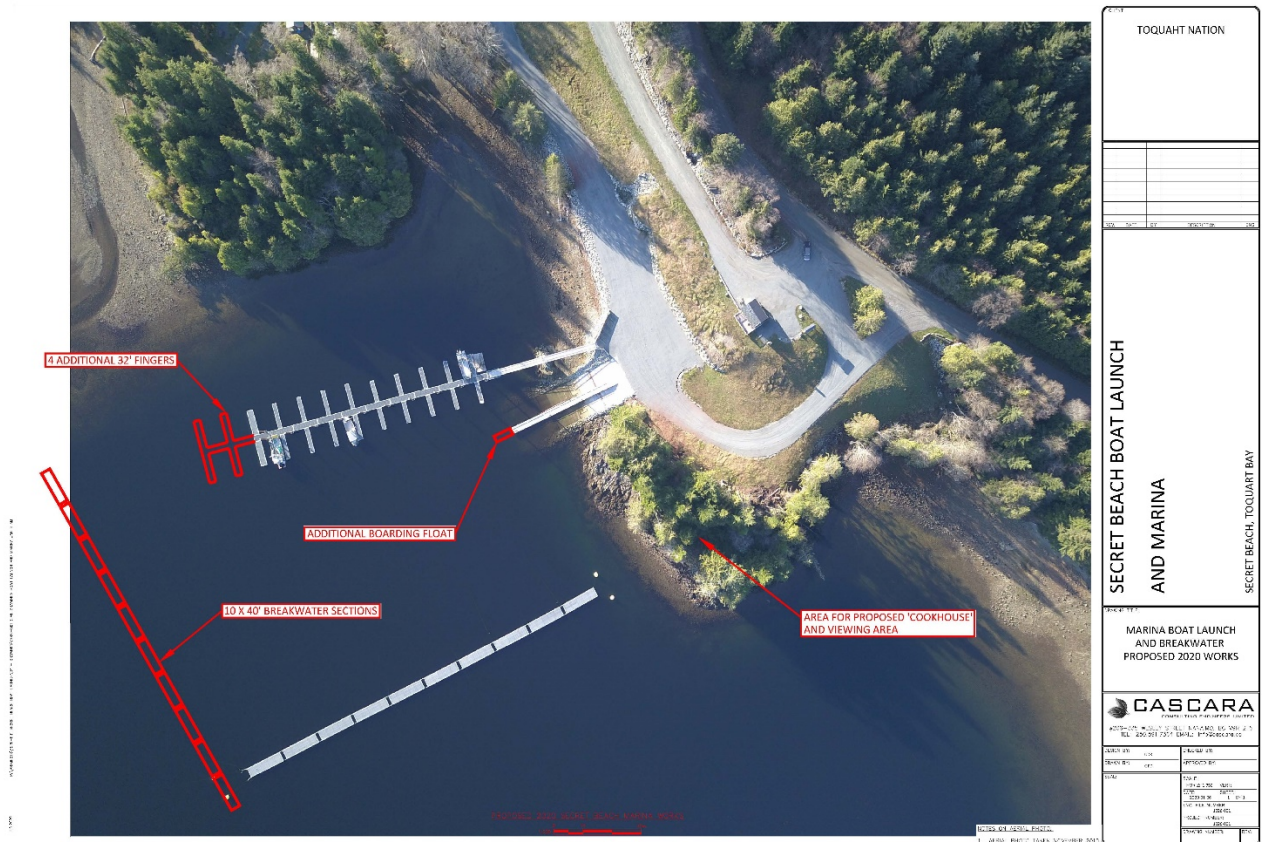
Air photo of Secret Beach Marina, 20/21 additions shown in red
